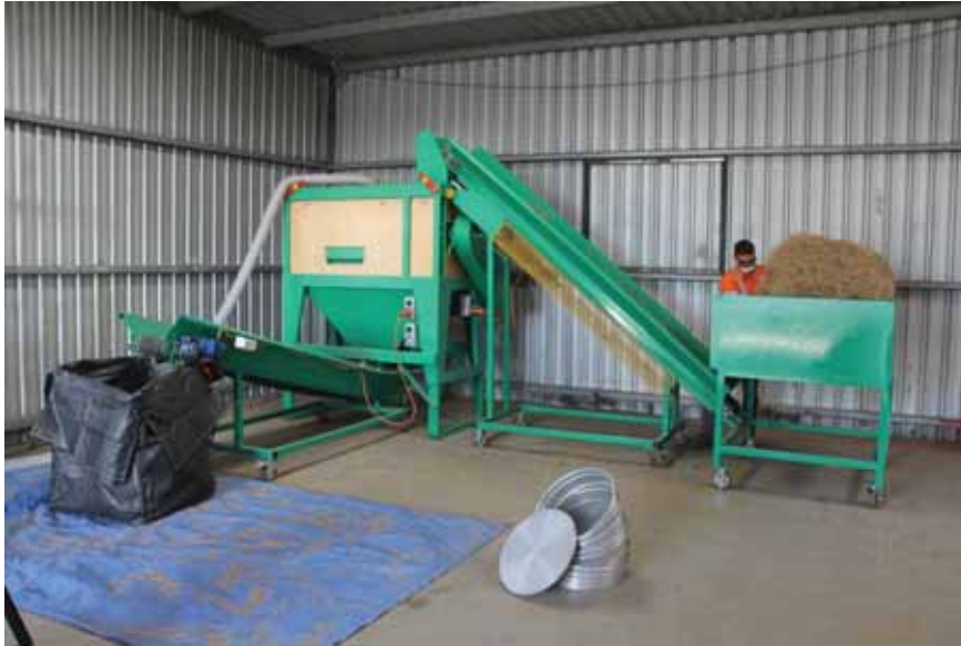
Figure 123: Native grass seed thresher used to process harvested seed into a form suitable for the direct-drill seeder.
