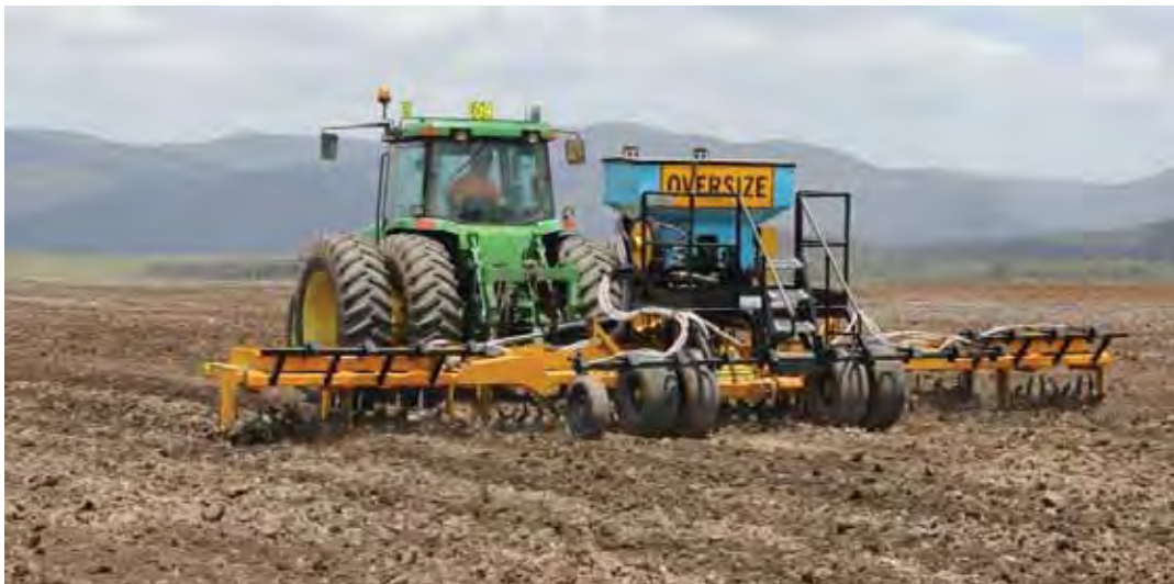
Figure 119: Aerator implement fitted with an air seeder used in 2014 to allow soil preparation and seeding to be undertaken in a single pass.
