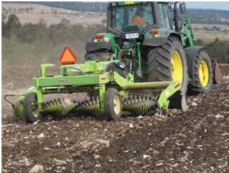
Figure 115: Rock windrower incorporating compost in rehabilitation, Cheshunt Pit
