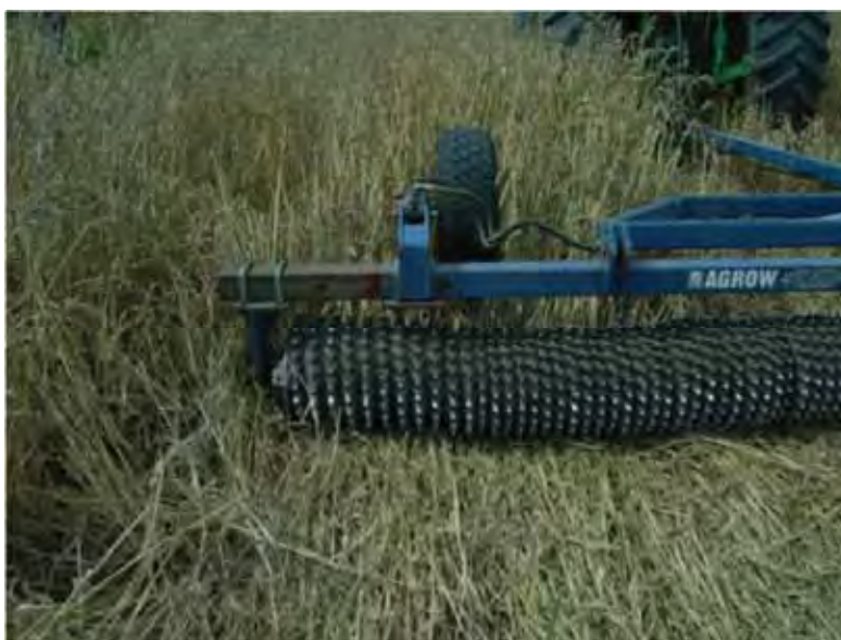
Figure 121: The flexiroller is made up of individual rings which allow it to conform to the surface contours
